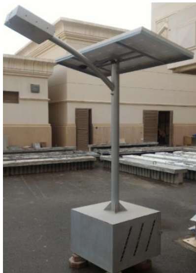
Figure 44: Solar system for the hydroponic.
