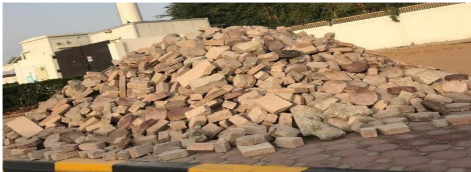
Figure 56: Used interlock provided by Sharjah Roads and Transport Authority.
